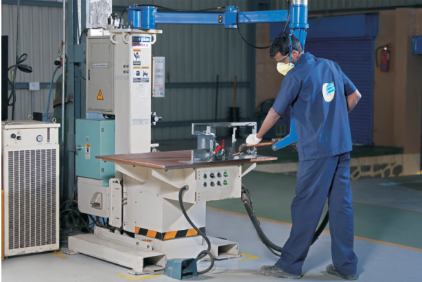
Special Table Top Type CNC Spot Welding M/c from Koyo Giken, Japan, a one-man operation
